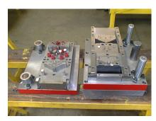
Custom Tooling & Dies built to Customer Specification. Progressive Dies to 10 ft. long & 6000 lbs. gross. Die Repairs, Sharpening & Engineering Changes.
